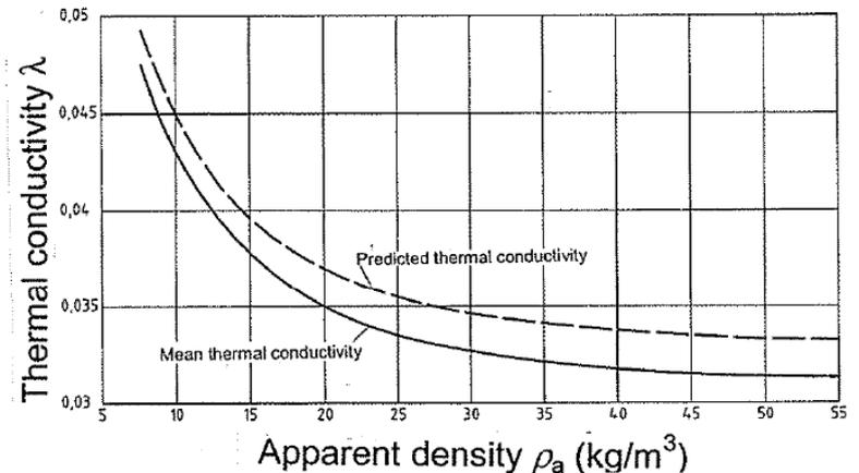
Figure B.2 — Relationship between declared thermal conductivity (at 50 mm reference thickness) and apparent density;  $1 - \alpha = 0,90$ ;  $n = 3873$
